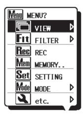
Move the cursor with the **UP/DOWN Keys** or **Shuttle Switch**, and confirm the selection with the **ENTER Key**. Pressing the **ESC Key** while the Menu is being displayed closes the Menu Window. Items displayed with "p" mark are accompanied with submenus. Press the **ENTER Key** to access to the submenus.
