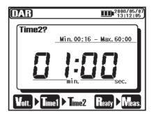
Setting items for DAR measurement are as follows. Refer to the Setting for Measurement (=>P.30) and change settings.
